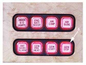
Note: The Generator uses the same fuel tank as the coach engine. The fuel pick up will stop drawing fuel at 1/4 tank, and will pull in air. Be aware of the diesel fuel level in the tank.
