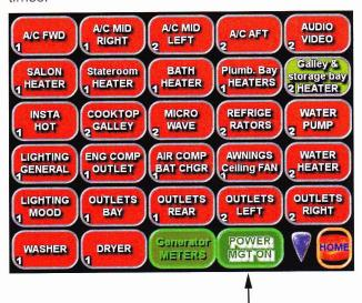
During periods of "Dry Camping" when you are "Inverting" and need to operate specific loads, you can turn the loads on, even with the Power Management activated (on). Good Load Management must be practiced to not exceed 35 amps per Inverter (while Inverting).
